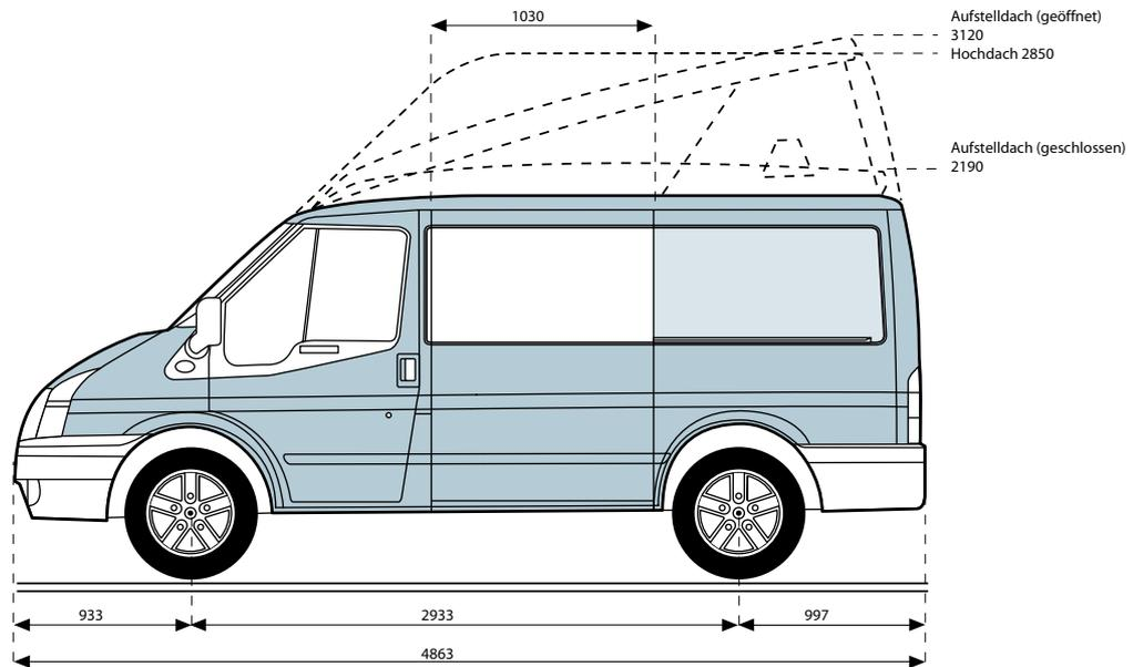
Abmessungen in mm, Ford Transit Nugget, kurzer Radstand
